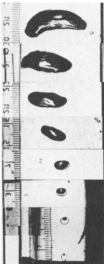
FIG. 16. Pentane drop evaporating in water (S12).
